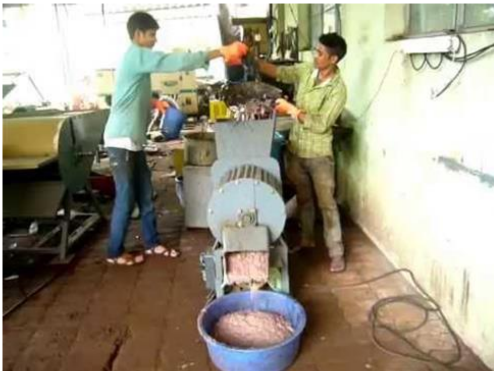
Figure 7. Fish rubbish grinding machine for preparing fish feed.
