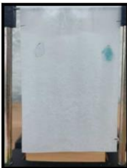
Figure 4. Ni 2+ and Co 2+ separation using paper chromatography by 3% NH 4 OH solution
