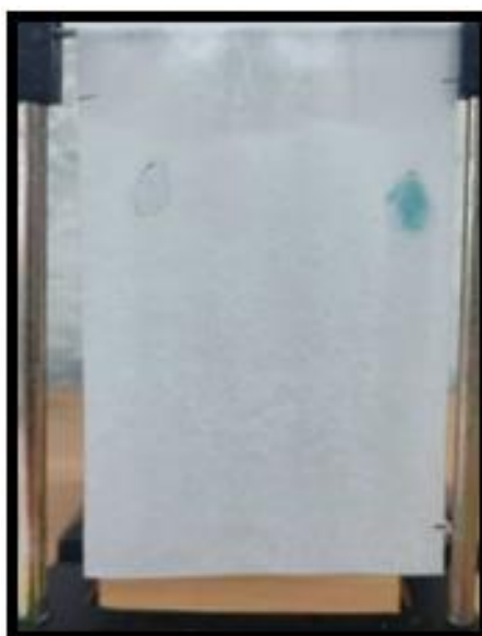
Figure 4. \text{Ni}^{2+} and \text{Co}^{2+} separation using paper chromatography by 3% \text{NH}_4\text{OH} solution
