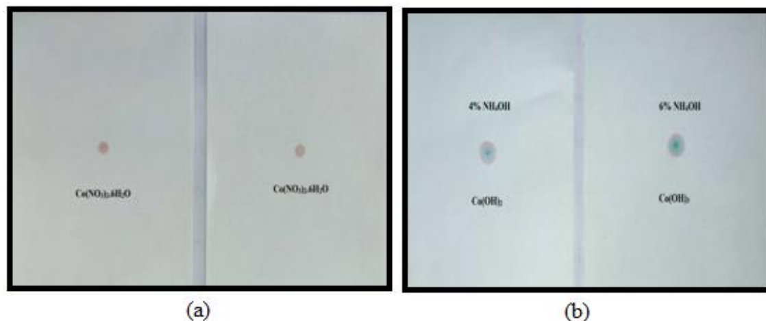
Figure 6. \text{Co}(\text{NO}_3)_2 \cdot 6\text{H}_2\text{O} spot detection within the Whatman chromatography strip (a) prior to and (b) with the addition of 4% and 6% \text{NH}_4\text{OH} solution
