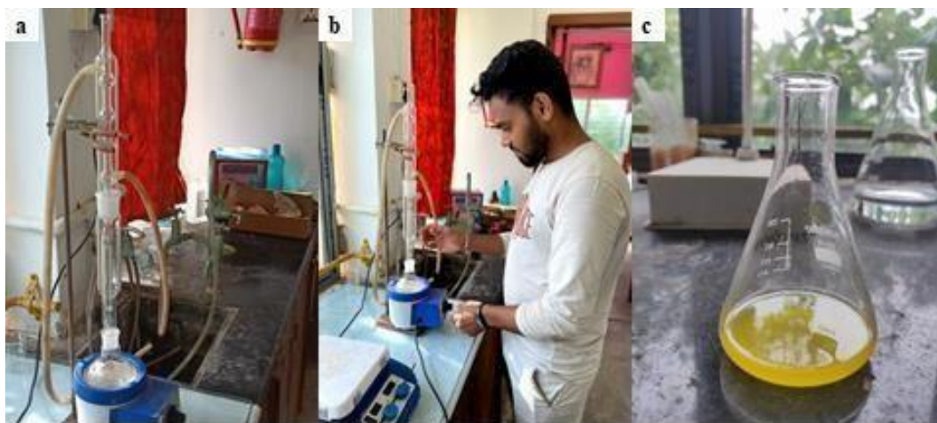
Figure 3. Extraction of oil using Soxhlet apparatus.
